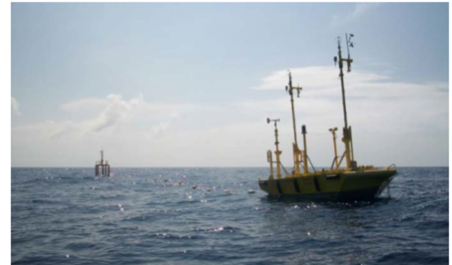
EASI-ASIS Buoys in tandem mooring
