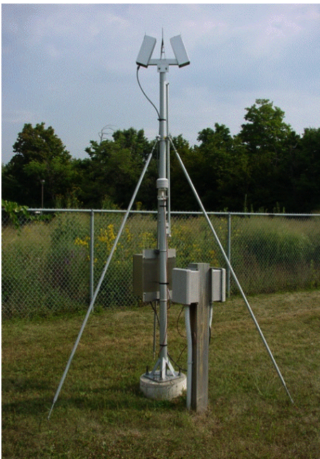
Fig. 3: (a) Precipitation Occurrence Sensor System (POSS) and (b) POSS Sensor Head Block Diagram.
